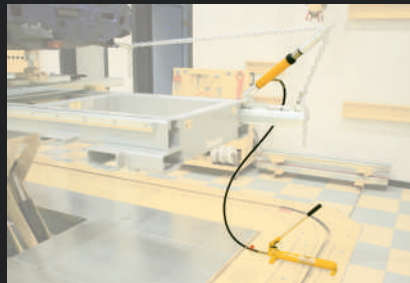
10T manual pulling kit for telescopic arm
