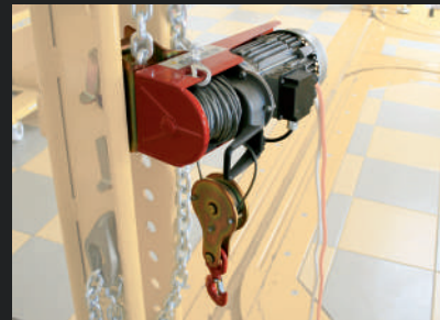
Electric winch (0.37kW-0.75kw motor)
